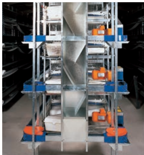
Cascade feed column prevents feed bridging
